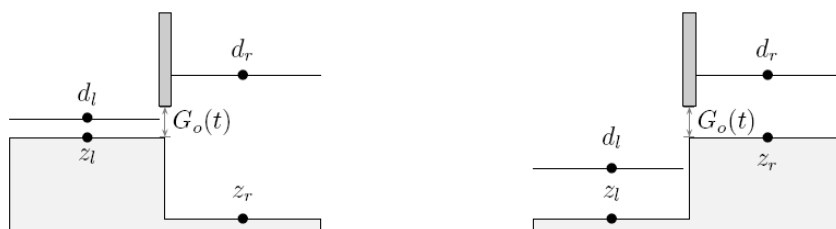
Figure 13.17 – Water levels for discharge under a gate in submerged conditions formulated as in (G2).
