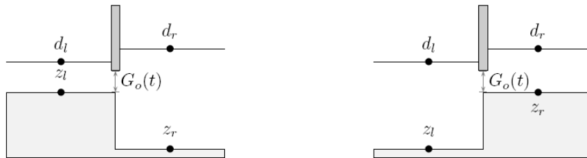
Figure 10.17 – Water levels for discharge under a gate in submerged conditions formulated as in (G1).
